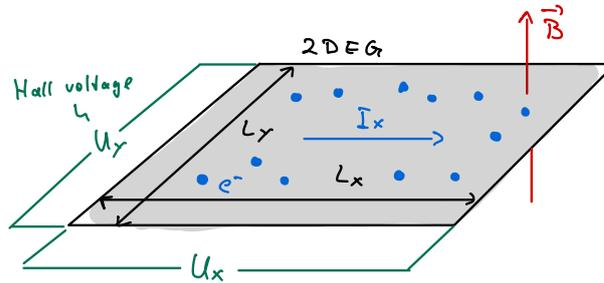
Our sample is wired such that a current  $I_x$  can flow from a connection on the left boundary to a connection on the right boundary (there is no source/drain on the boundaries in  $y$ -direction,  $I_y = 0$ ). There are voltage probes on all four boundaries to measure the voltages  $U_x$  and  $U_y$ .
