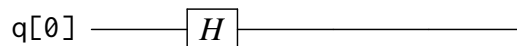
Figure 10.7 Quantum circuit for the simulation of a single Hadamard gate on one qubit.
