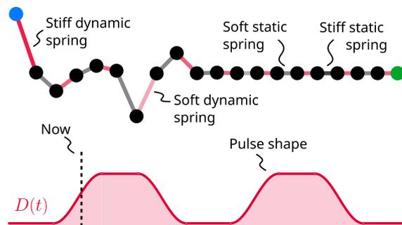
We color static (tunable) springs in shades of black (red). The shape of  $D(t)$  is plotted below the pendulum chain; the current point in time is marked by a vertical line in this plot.
